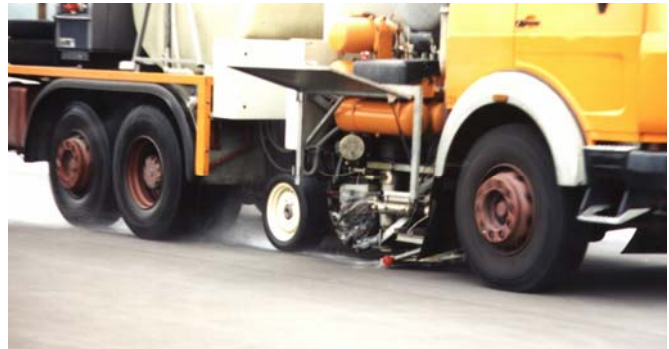
Measuring skid resistance by means of the Universal Skid Resistance Measurement Device (URM II) of FKFS
