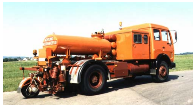
Stuttgart Skid Resistance Measurement Device (SRM) of FKFS
