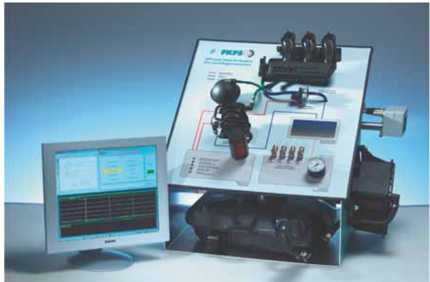
Demonstrator for a model-based leakage diagnosis of a fuel tank without additional sensor systems
